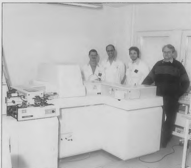
The VG Autospec tandem mass spectrometer and several members of the Glyco- and Transplantation Biology Group. From the left, Drs Steve Henry, Sohbat Ghardashkani, Mikael Gustavsson and Professor Bo Samuelsson. Mass spectra are recorded on this hybrid tandem instrument with a magnetic sector as MS-1 and an orthogonal time-of-flight device as MS-2 (AutoSpec-TOF, VG Analytical, Manchester, UK).
